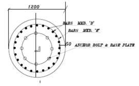
Fig 16. Typical Cross Section of Pedestal
