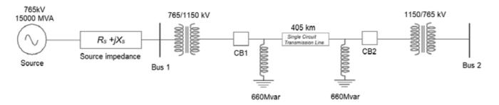
Fig.1 Schematic of 1200kV UHVAC system
