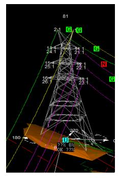
Fig 11: Tower at location number 81 with leg extensions on TIN ground profile
