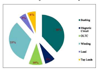
Fig. 1. Component Wise Failure Causes
