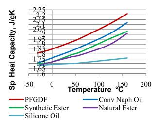
Fig. 4: Specific Heat Capacity of DFs
