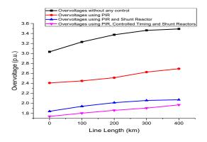
Fig. 10: Comparison of Overvoltage magnitudes for different methods
