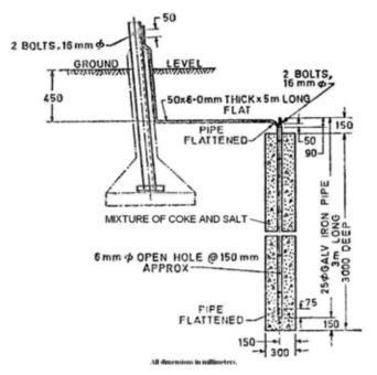
Fig 12 Pipe Grounding (Treated) Specified in India
