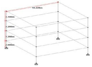
Fig 6. STADD model of column and tie beams for 9.5 m RC.
