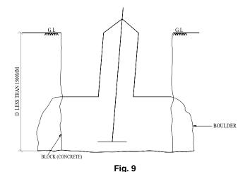
The location of tower on hard rock should be selected away from the vertical cliff to avoid blasting off the excavated pit in the valley or exposure of foundation due to weathering.
