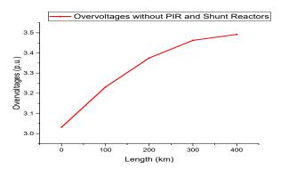
Fig 3: Variation of Overvoltages at various lengths of the line without using any mitigation method
