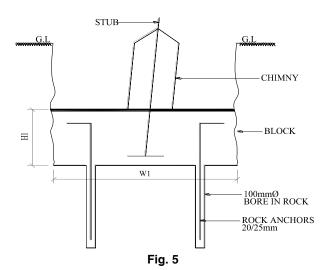
If the holes are not drilled with the desired diameter 'd' and the desired depth 'D', there are chances of premature failure of foundation against the upward force.
