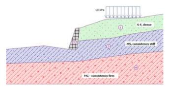
Fig 16: Typical slope stability study assignment
