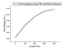
Fig 7: Variation of Overvoltages at various lengths of the line using both PIR and Shunt Reactor
