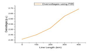
Fig 5: Variation of Overvoltages at various lengths of the line using only PIR
