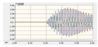
Fig 2: Overvoltage waveform when no control is used
