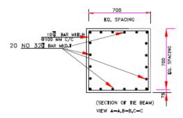
Fig 15. Typical Cross Section for Tie Beam
