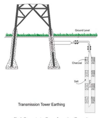
Fig 9 Transmission Tower Grounding (Treated)
