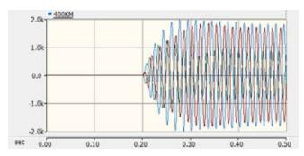
Fig 4: Overvoltage waveform when only PIR is used
