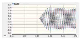
Fig 8: Overvoltage waveform when PIR with controlled switching and shunt reactor is used
