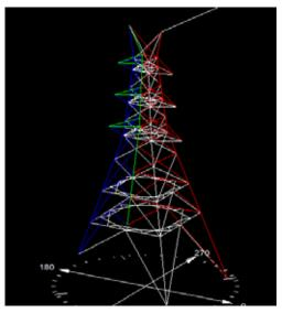
Fig. 6: DB+0 Type of towers with actual leg extensions
