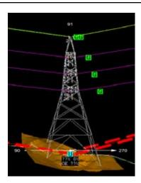
**Fig 12:** Tower at location number 91 with leg extensions on TIN ground profile
