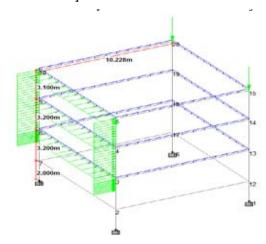
Fig 7. Vertical loads on beams
