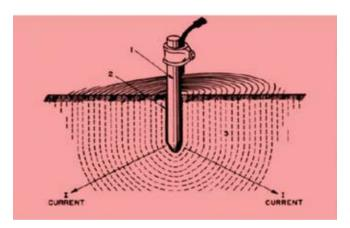
Fig 5 Different Components of Grounding Resistance
