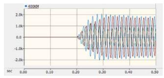
Fig 6: Overvoltage waveform when both PIR and Shunt Reactor is used
