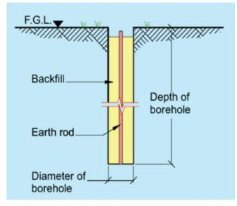
Fig 7 Concept of Chemical Grounding
