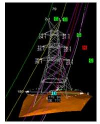
Fig 10: Tower at location number 79 with leg extensions on TIN ground profile
