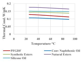
Fig. 3: Thermal conductivity of DFs
