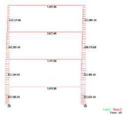
Fig 12. Shear Force Diagram
