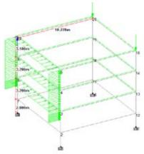
Fig 10. Uplift and compression loads pedestals in Vertical direction
