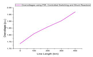
Fig 9: Variation of Overvoltages at various lengths of the line using PIR with controlled switching and shunt reactor
